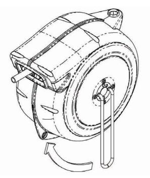
Note: Never add or remove tension when the hose is extended from the reel. The hose must always be fully wound on the hose reel.
